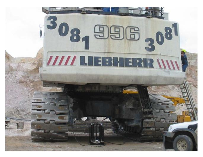
Griffin Coal contacted Equipment Placement, Filter Technology Australia's representative in Western Australia. They constructed a mobile unit to do the job while the machine was on a programmed shutdown. The shutdown allowed only 12 hours to circulate the 4,000 litres in the hydraulic system.
