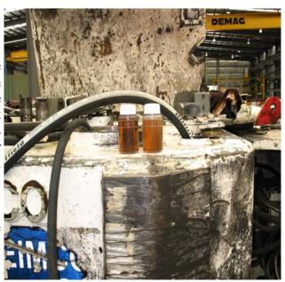
The oil analysis attached indicates the oil before filtering was at an ISO 19/13 and after eight hours the after sample indicates an ISO 12/9 a reduction of 96% in particulate contamination.
