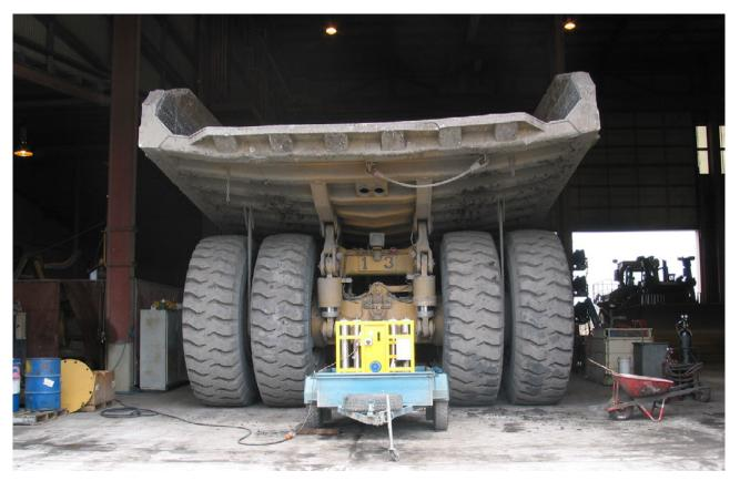
This time the unit chosen was a FM1640 fitted with a 20 litre per minute pump. The finaldrive housings have been drilled to allow oil to flow from the hubs to the centre of the finaldrive, pipes were fitted in a recent overhaul which allowed the oil to be sucked from the right hand side hub and returned to the left hand side hub, quick release couplings were fitted to the inspection plates that enable ease in hooking up the kidney unit. (As in picture)
