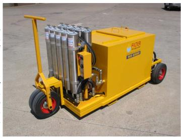
The oil report below indicates the 600 litres of oil out of the drums was at ISO 22/18 and after four hours kidney looping through the FM1040T the oil was delivered to the finaldrive at ISO 15/11 a reduction of 89% in particulate contamination, the microscopic patches give a better understanding of the amount of contamination that has been removed from the oil.
