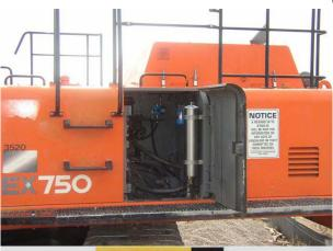
The system was re sampled at 1443 hours 63 hours after installing the KS-100-A-FM3. The report below indicates the oil now at 18/15/13 at reduction of 94% in particulate contamination, copper reduced 5 ppm which indicates these particles are sub micron level.
