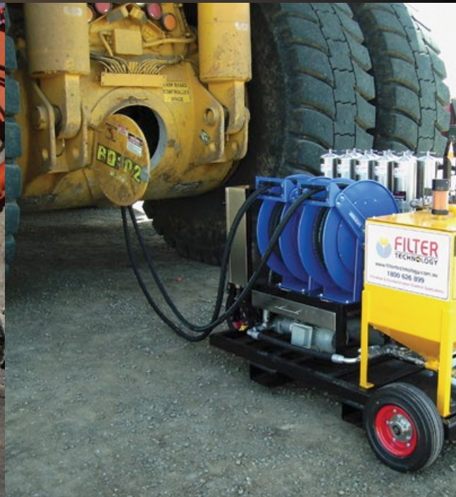
Kidney loop filtration on final drive unit using mobile filtration buggy
