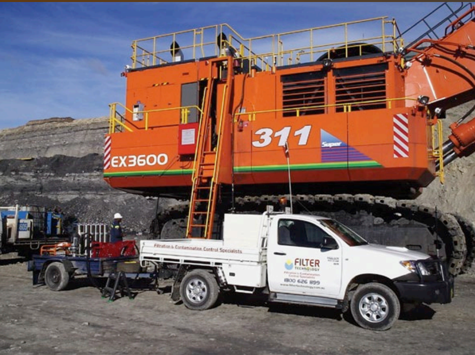
Trailer mounted units enable kidney loop filtration to be carried out on-site.
