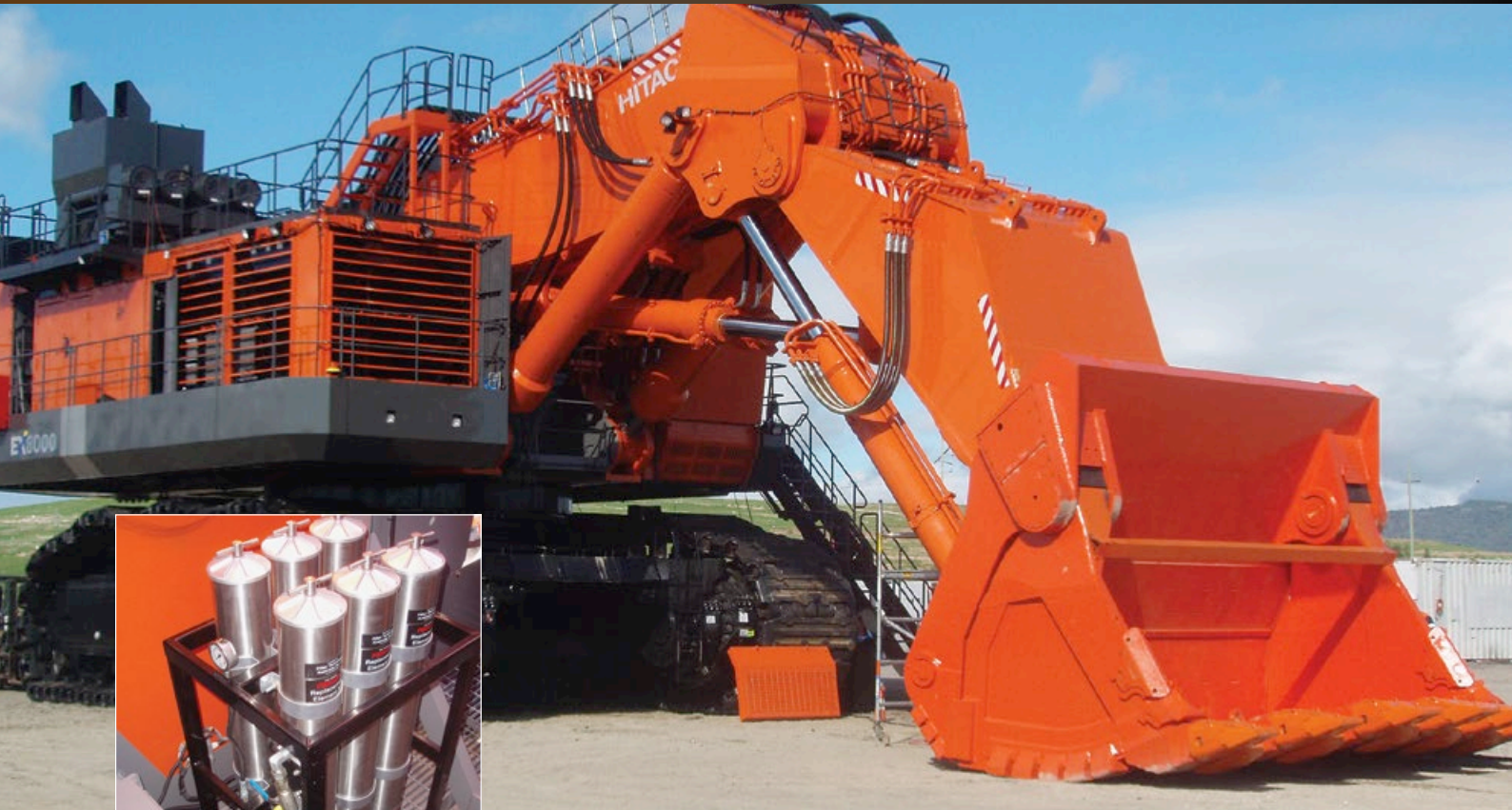
On-board filtration systems for industrial oil extend fluid and component life dramatically
