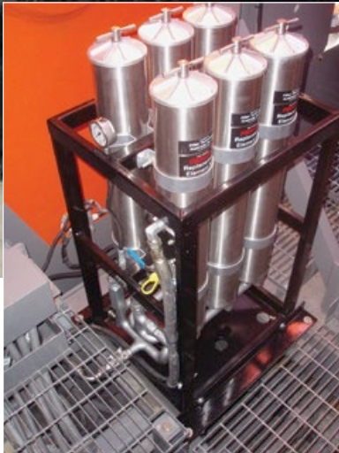
On-board filtration systems for industrial oil extend fluid and component life dramatically
