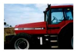
Since fitting the filters the tractor has stopped using oil and the owner says it is performing better. He has set a benchmark of 750 hours on oil changes, up from 250 hours. Using oil analysis has helped set the trends for servicing.
