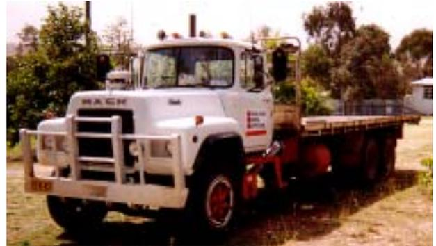
In using oil analysis to trend, the above goals have been achieved and samples indicate the oil at 80,000km having lower iron and soot levels. Consequently, 80,000km has been set as a benchmark for future oil changes. Filter Technology elements are changed at 25,000km and 5 litres of top-up oil is added.
